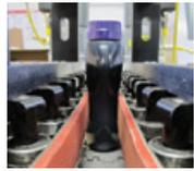
As a container passes through the system, dual parallel belts apply force to the sidewalls of the container. This action compresses the headspace of the container which allows a sensor to take a force measurement at the discharge of the system. Utilizing DSP technology, the controller analyzes the measurement and assigns a merit value to each container. If the merit value is outside of the acceptable range, a reject signal activates a remote reject system.
