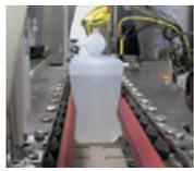
The system is designed with dual parallel belts suspended over the customer's existing conveying system. As the container passes through the system, the dual parallel belts apply force to the sidewall of the container. This action compresses the headspace of the container that allows a comparative measurement to be taken at both the
