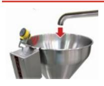
Photo Sensor monitors product level in the hopper and controls the pump
